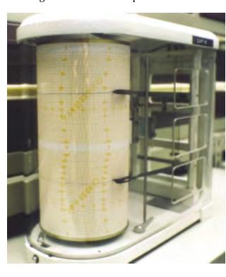
The hygrothermograph produces a continuous record of relative humidity and temperature
