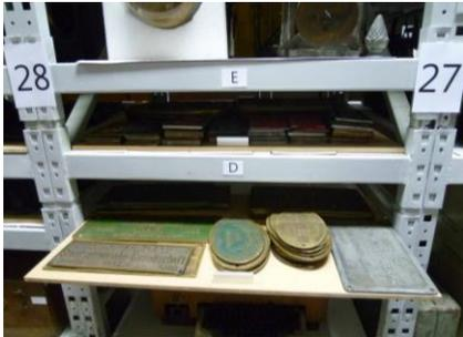
**Sliding plywood boards** on shelving are simple and cheap for storing objects flat © ICCROM
