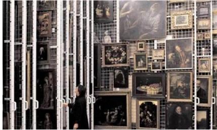
**Sliding racks** take up less space; works are fully visible, but the cost is high © ICCROM
