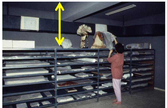
Clear height, or usable vertical space, is not always the same as the room height because of various obstructions (in this case, ventilation ducts) © ICCROM
