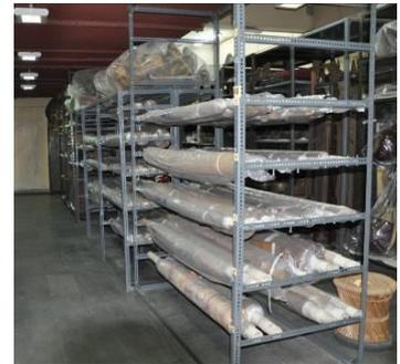
**Modified shelving units** fitted with horizontal bars to support tubes © ICCROM
