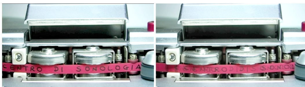
FIGURE 3. Test for video shooting. On the left, a correct setting of the camera: each frame is clear and the text is readable. On the right, a wrong setting of the camera. The aim is to detect physical defects of the tape (due to aging or joints) that may correspond to a specific noise in the audio signal. Audio is directly recorded from a secondary output of the STUDER A810.
