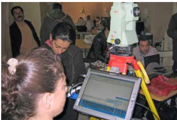
Fig. 4. Using the total station with a tablet PC. Photo by Robin Letellier.
