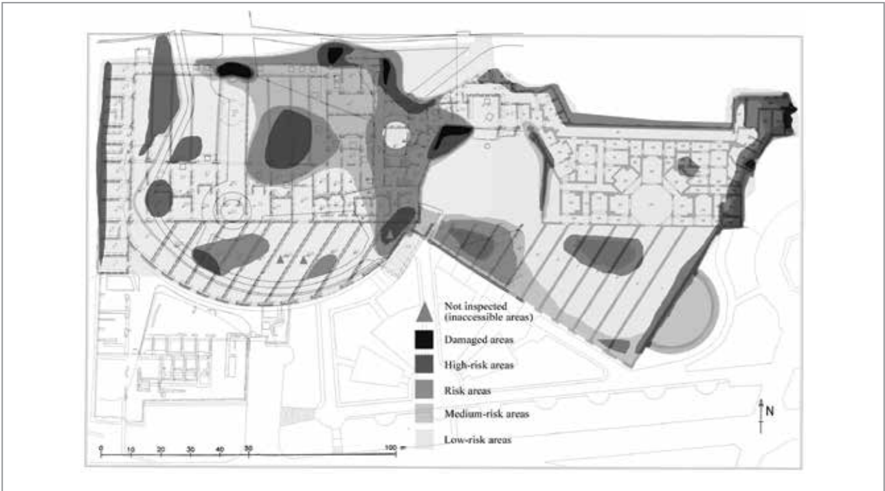
Fig. 2. A risk map of damage caused by tree cover, including potential extension of roots, over the subterranean remains of the Domus Aurea, Rome, (© Giulia Caneva; from Caneva & Ceschin 2006)
