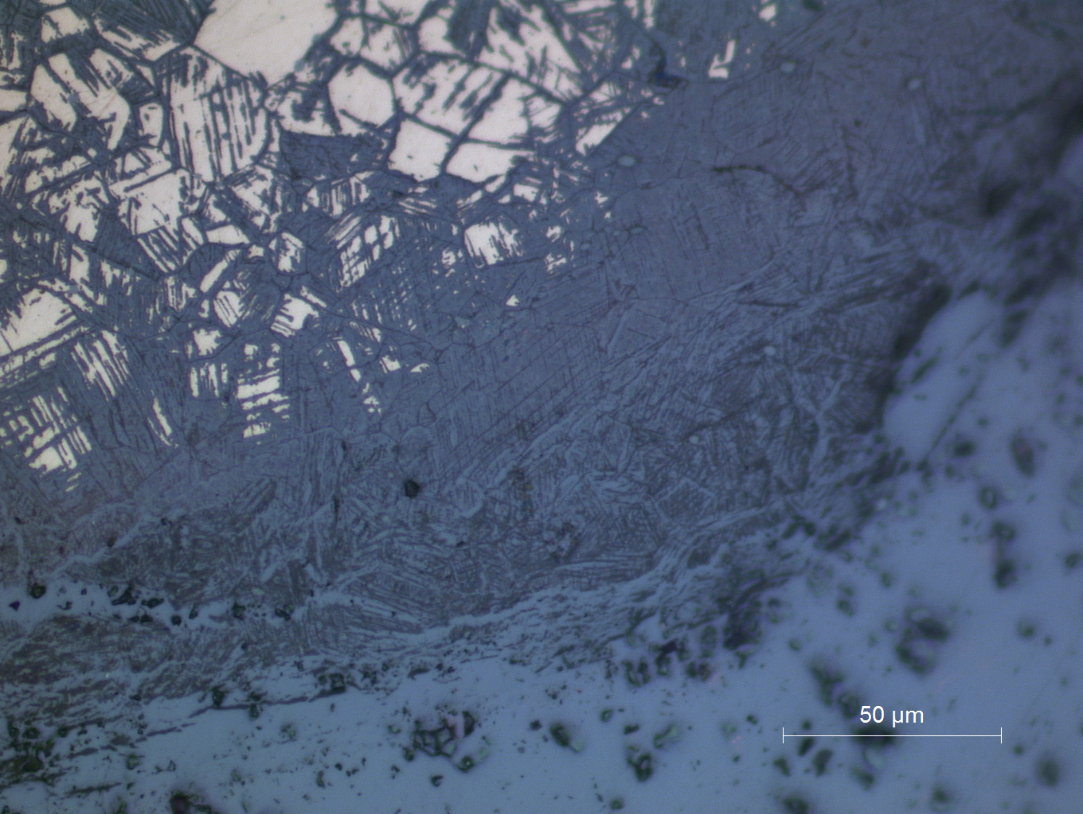
A159.3 Detail to show flow and strain lines in the inner side of the corrosion products.
