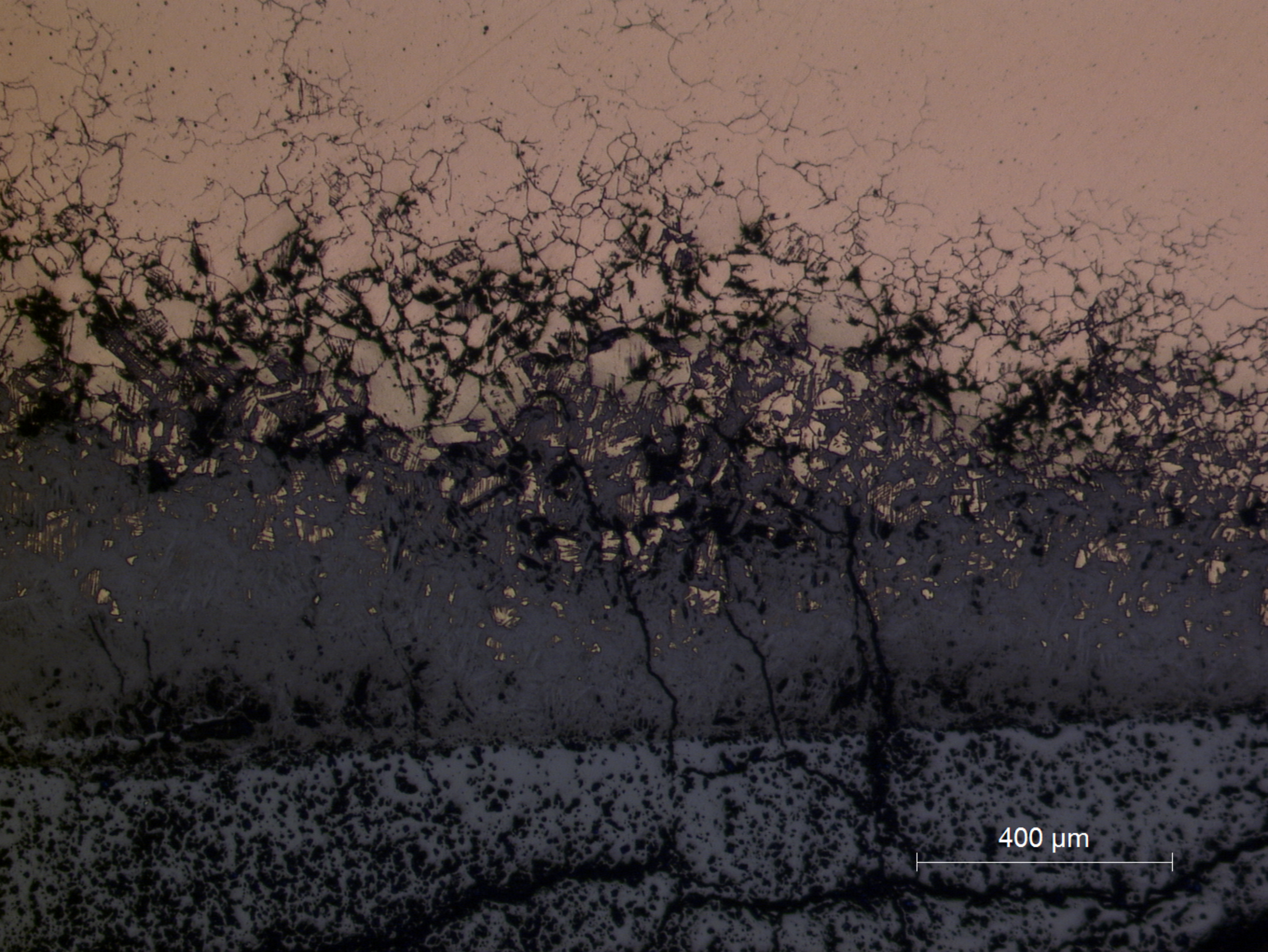
A159.1 General view near the surface in which can be seen the metallic core in the upper part (white); a zone of progressive corrosion towards the bottom; the original surface (straight line); and the outer part of corrosion products.
