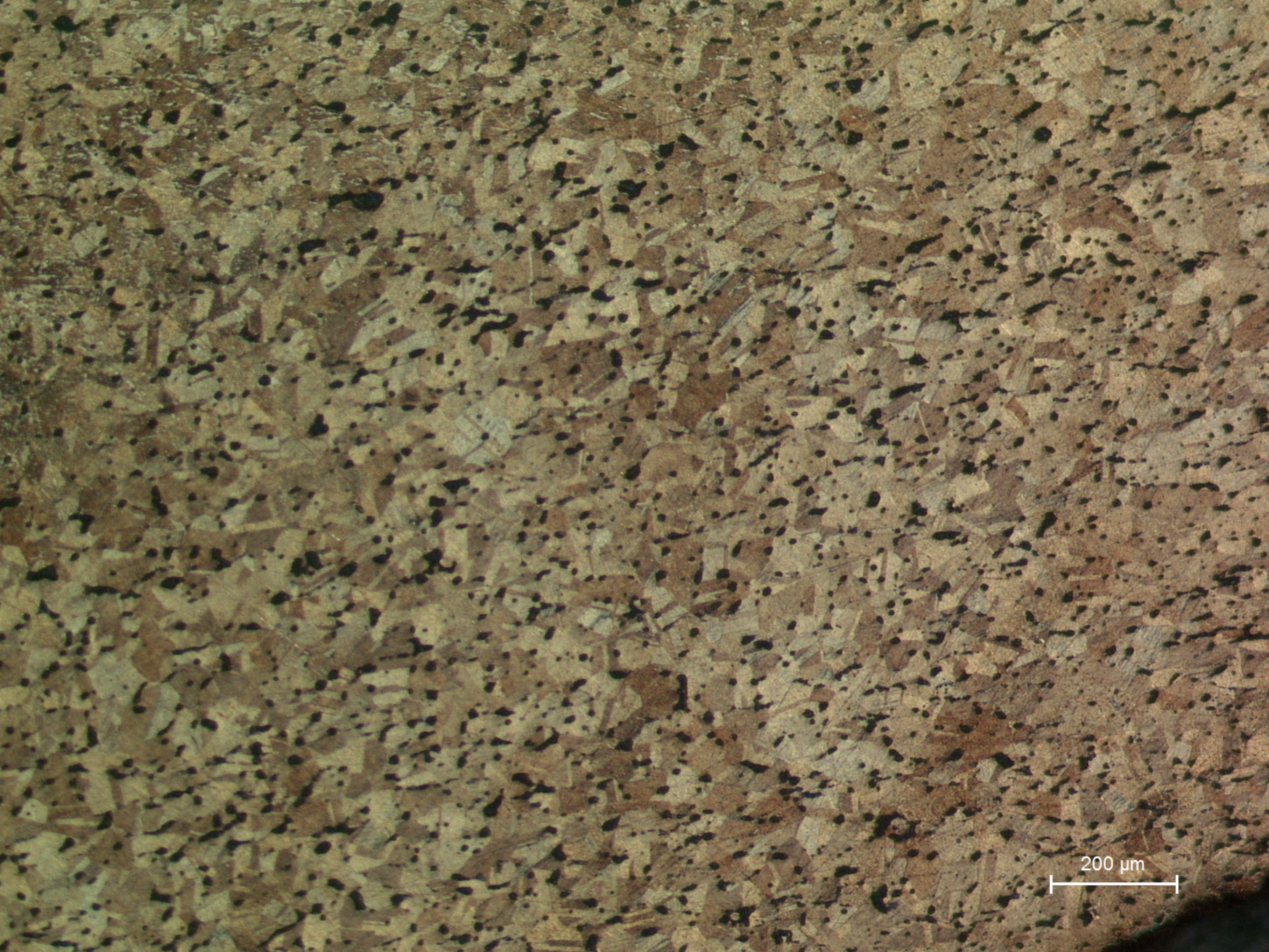
A183.1 General view showing slightly deformed recrystallized grains with annealing twins and a large number of inclusions (containing Pb, Zn and S) (etchant: aqueous \text{FeCl}_3 ).
