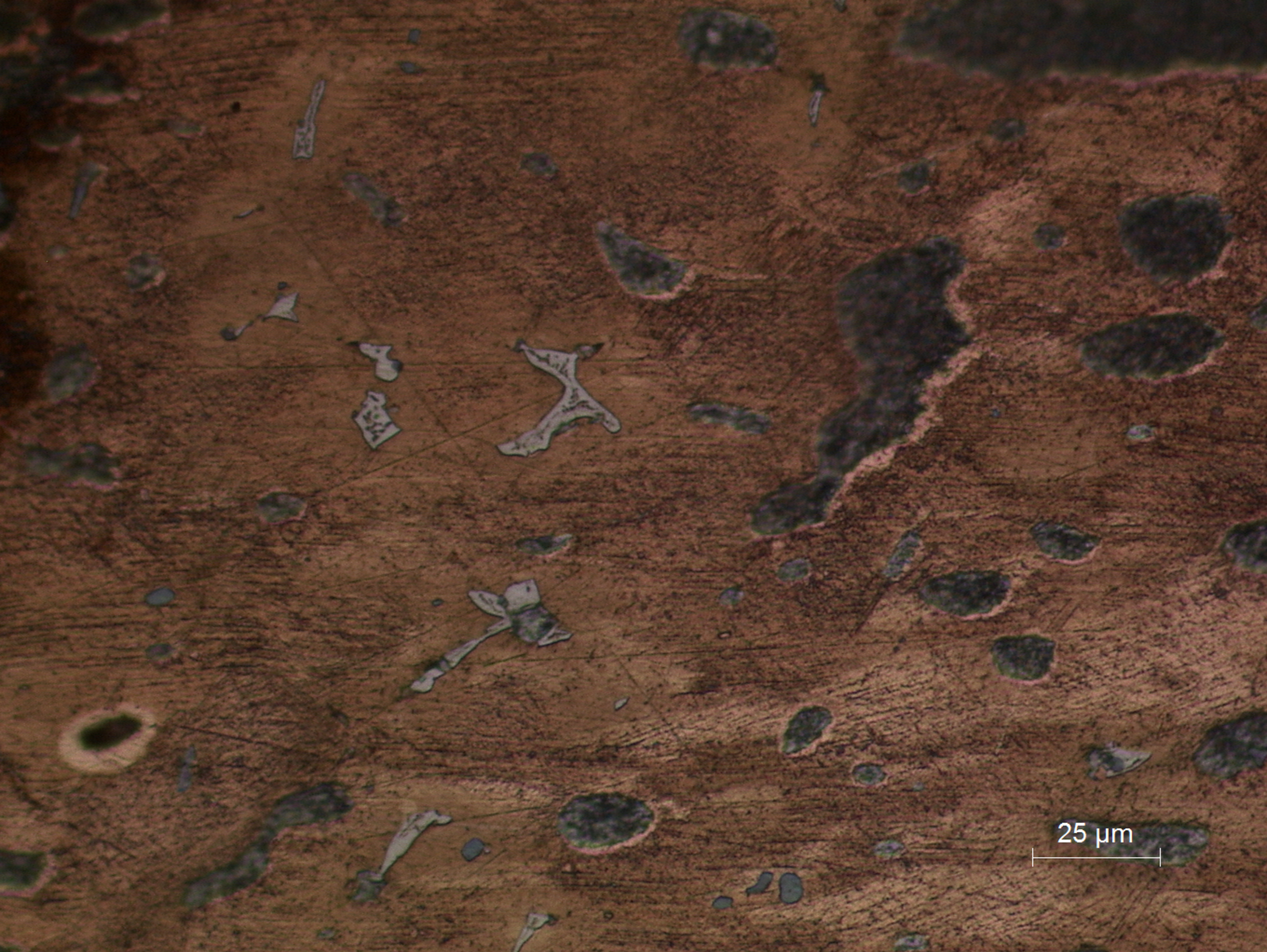
B07.2 Detail of the Cu-rich matrix with many Pb globules (dark grey) and a small amount of eutectoid phase (white); numerous sulfide globules (blue grey) (etchant: aqueous \text{FeCl}_3 ).
