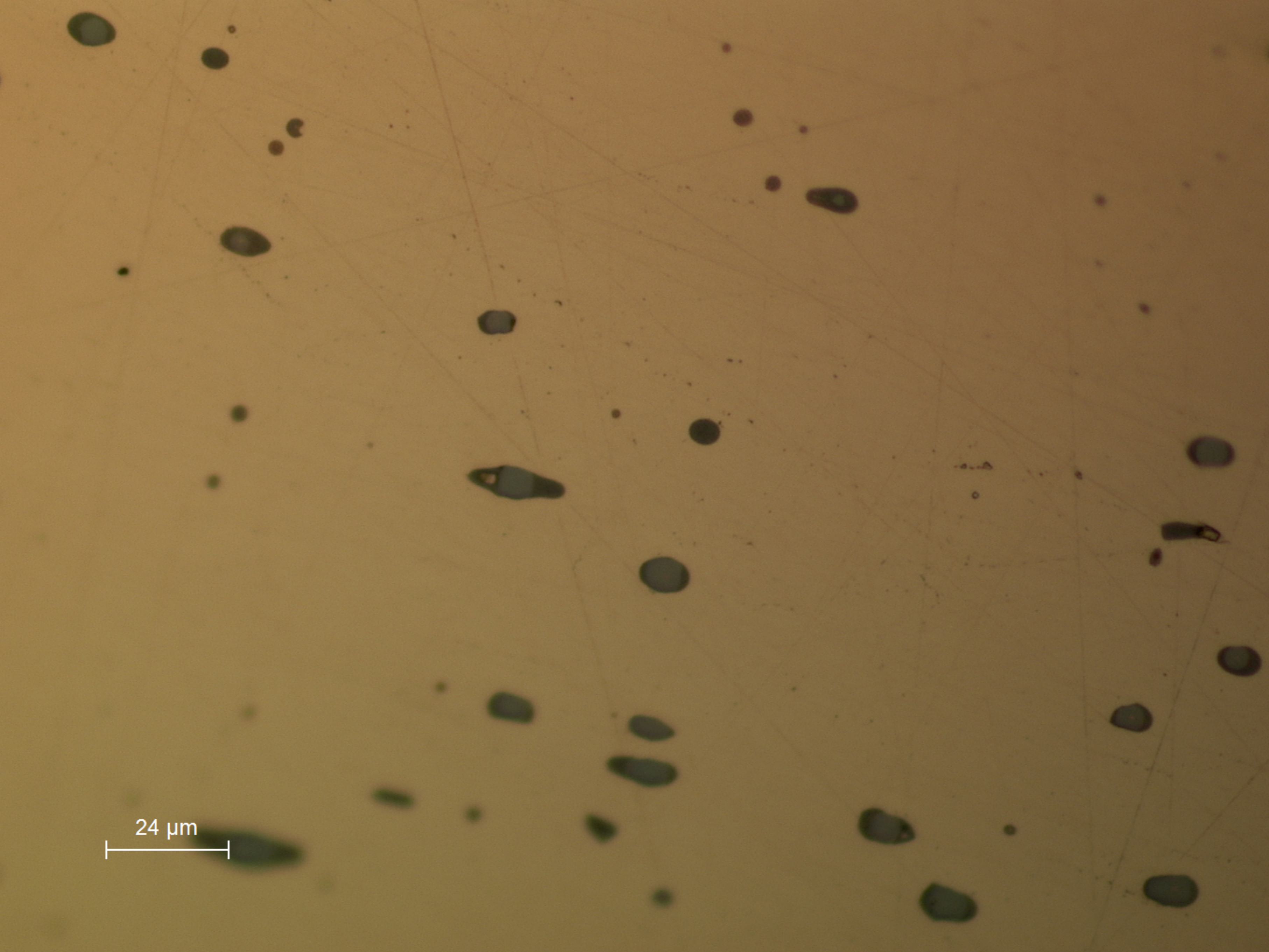
B22.3 Detail showing inclusions containing many phases, which are constituted by different elements: As, Sb and Pb.
