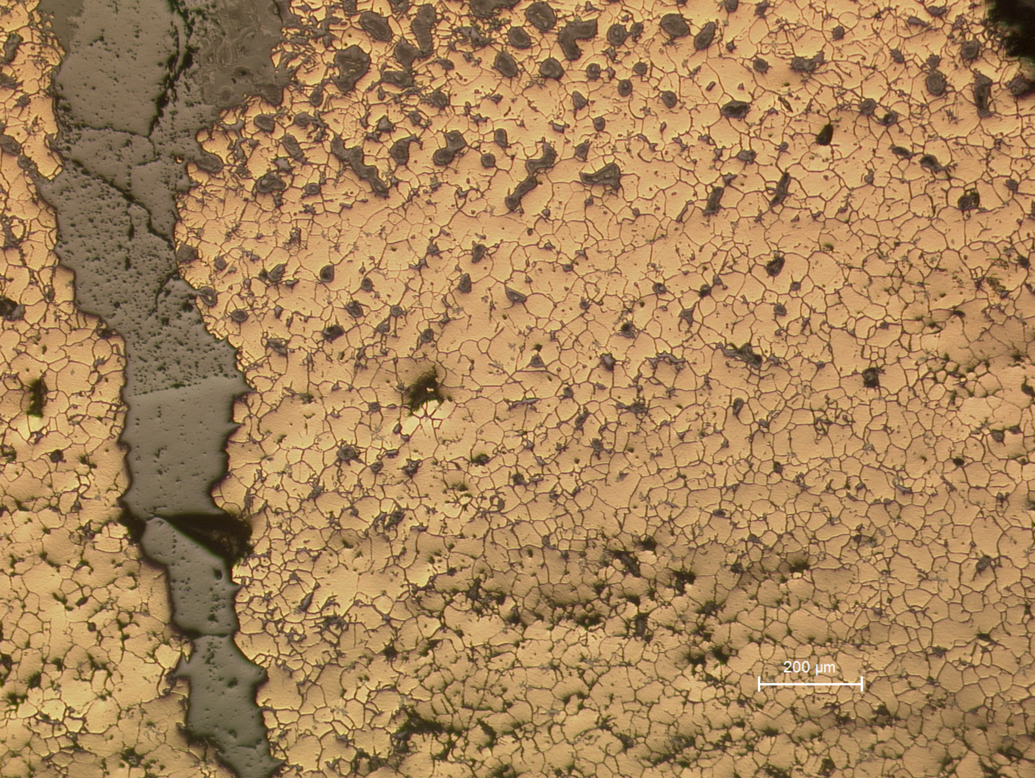
B93.1 General view showing the area near the surface (top) and a huge crack filled with oxides.
