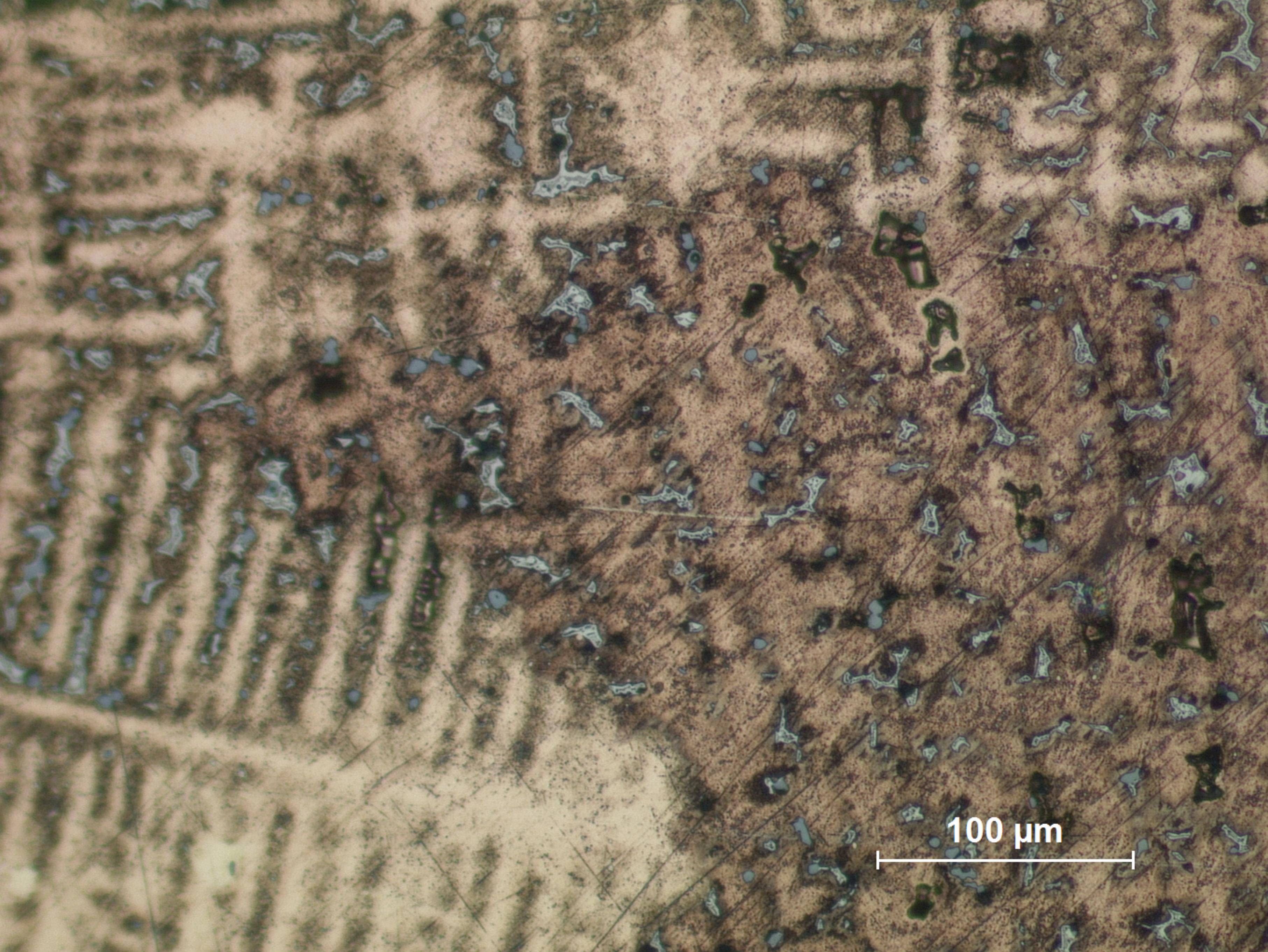
B95.4 Detail of the central part of B95.3, showing the interdendritic segregation of the eutectoid phase and inclusions (mostly sulfide and lead) (etchant: aqueous \text{FeCl}_3 ).
