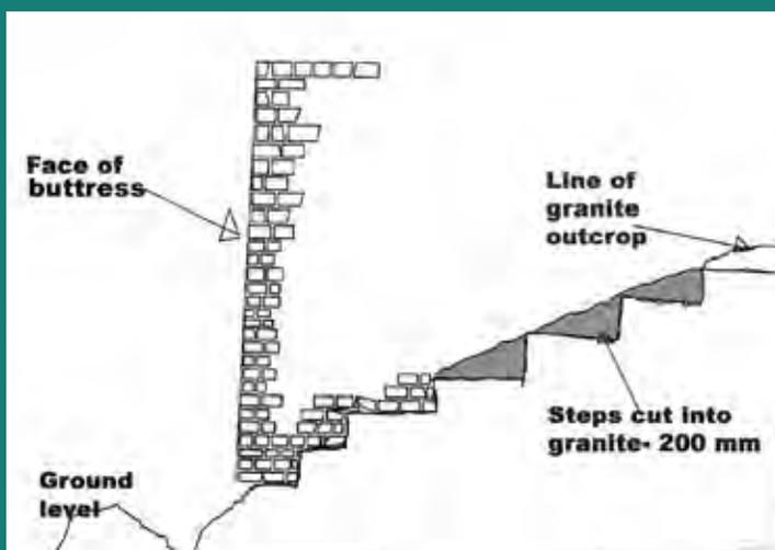
FIGURE 5.2 Steps cut into granite
