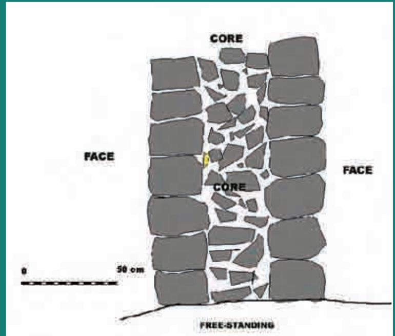
FIGURE 3.6 Illustration of the components of a free-standing dry-stone wall
