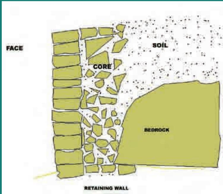
FIGURE 3.5 Illustrated dry-stone walling used for platform construction
