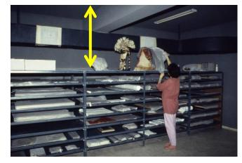
Clear height, or usable vertical space, is not always the same as the room height because of various obstructions (in this case, ventilation ducts) © ICCROM
