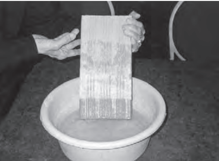
A practical example to explain the crystallization process. In a few days it is possible to see the concentration of salts on the brick and the beginning of the crystallization phenomenon.
