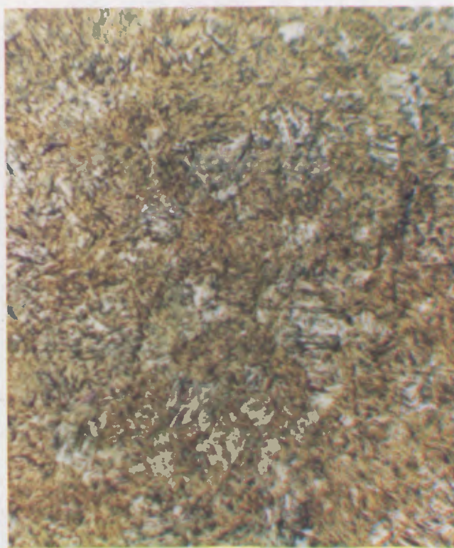
Fig. 63: The same steel heated to 870°C and then tempered in water. The structure has changed, it is now martensite, a very hard needle-structured component, a super-saturated solution of iron carbide in \alpha iron. Magnified \times .
