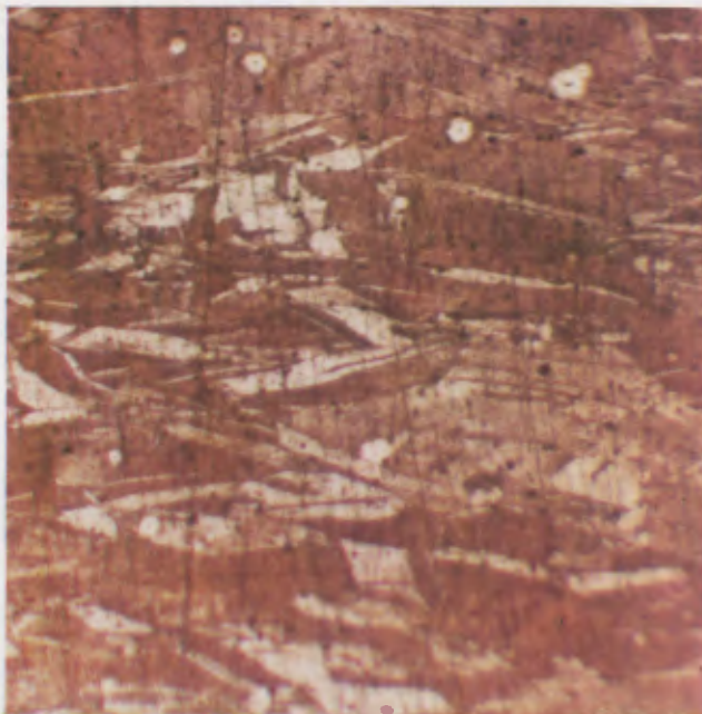
Fig. 24: Flattening of the grains in the direction of the hammering. Magnified 100 \times .
