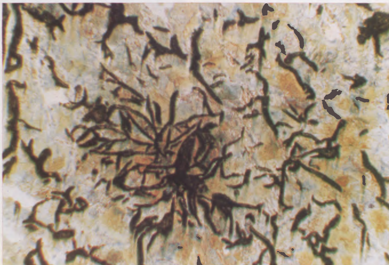
Fig. 60: Cast iron containing 2.93 % carbon; ferrite and carbon in the form of graphite and arranged in rosette patterns are in a pearlitic matrix. Magnified 200 ×.
