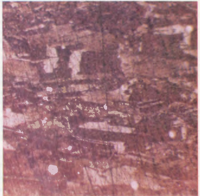
Fig. 27: The elongation of the grains is visible. Magnified 100 x.
