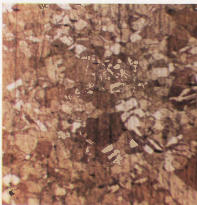
Fig. 22: Same section after reheating. The structure of the drawing has disappeared. Magnified 100 x.
