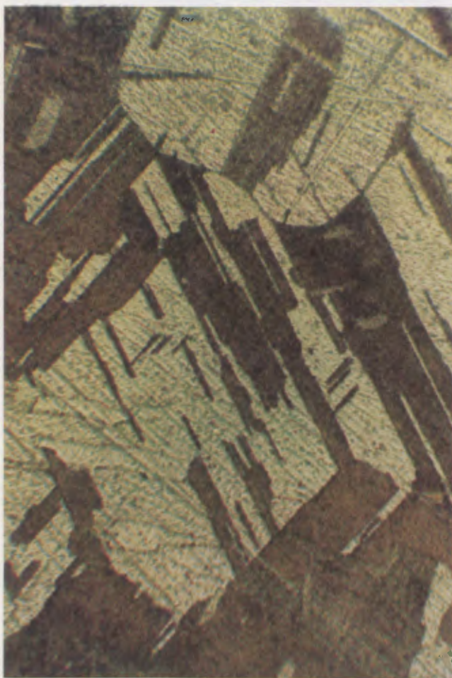
Fig. 33: Pure silver, cubic crystals, reheated metal with large grains. Magnified 200 ×.
