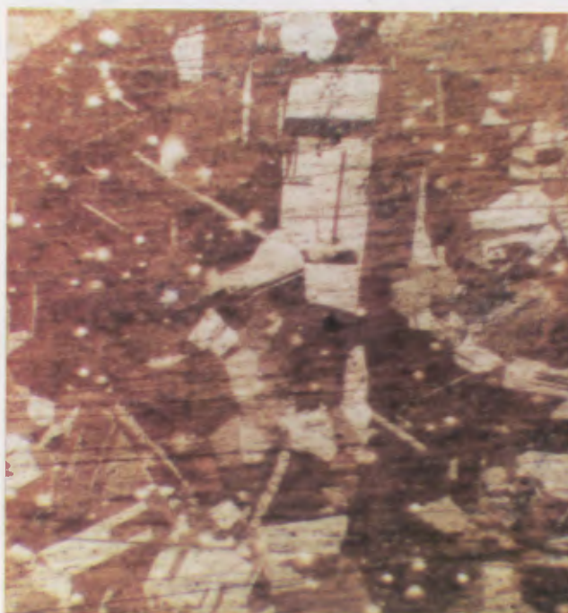
Fig. 19: Reheated until red hot and then left to cool. The grains appear. Magnified 100 \times .
