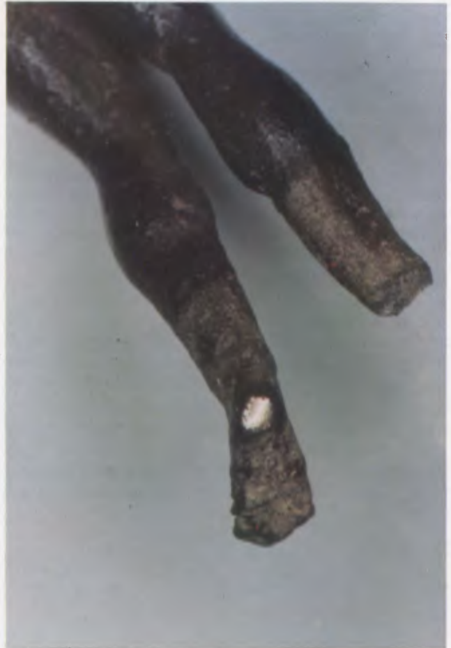
Fig. 75: Direct examination. A small surface area has been removed and several millimetres polished. Magnified 3\times .
