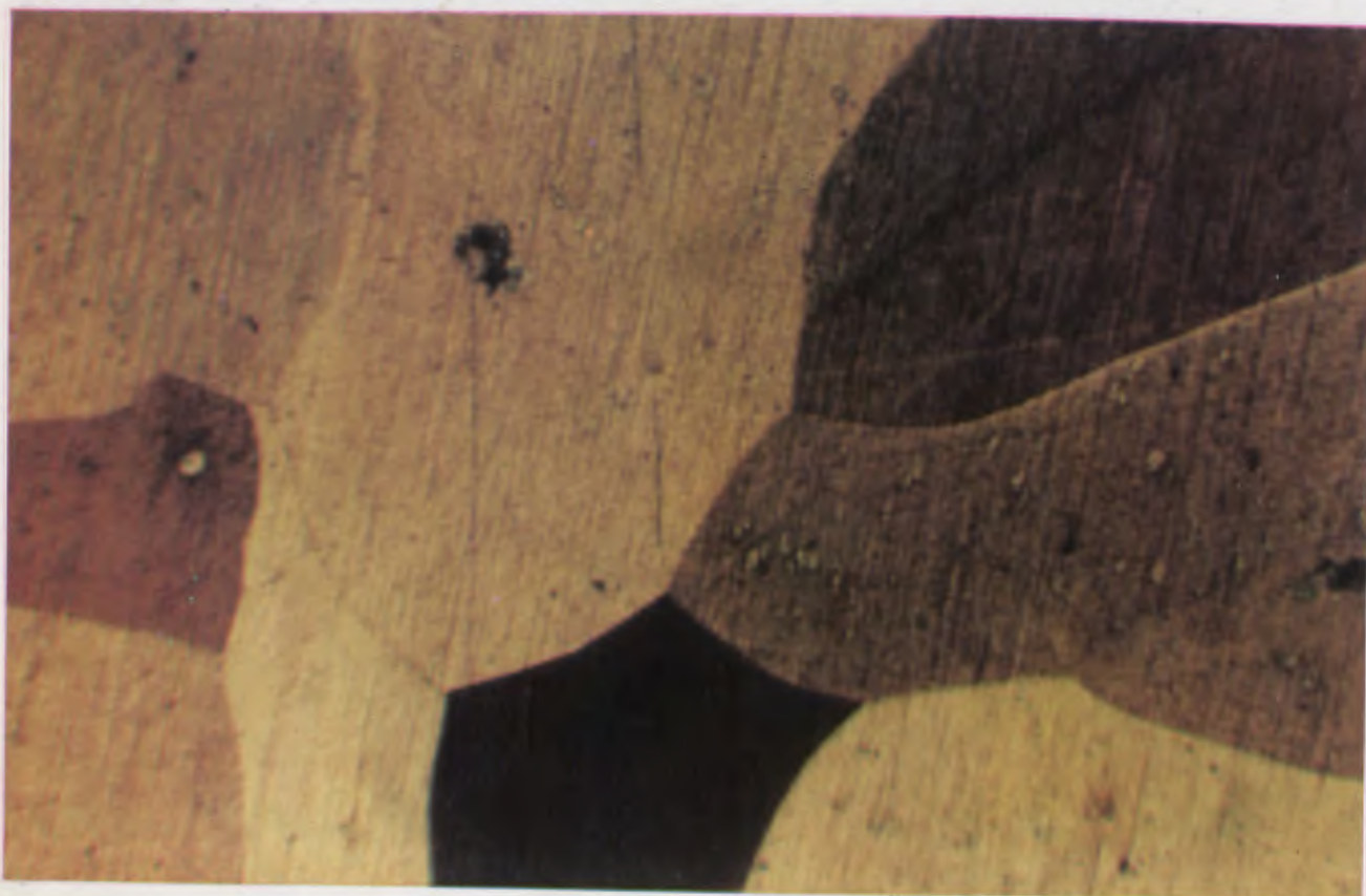
Fig. 11: Brass alloy obtained by sand casting. Large basaltic equiaxial grains. Magnified 100 \times .
