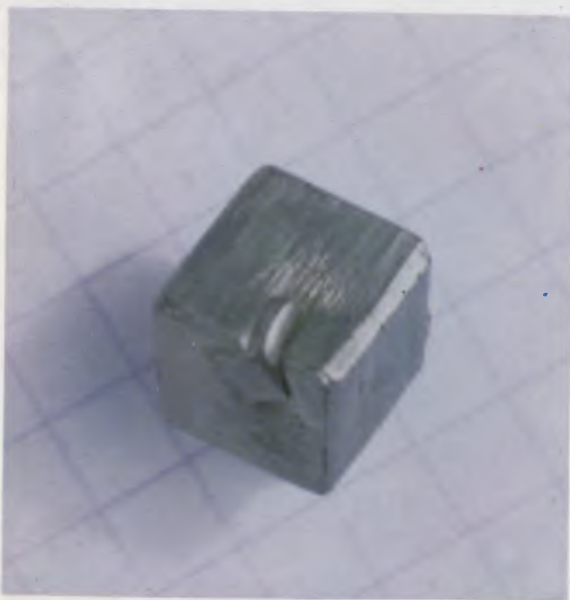
Fig. 9: Small cubic pyrite crystal, ferrous sulphide, \text{FeS}_2 . Magnified 1.5 \times .
