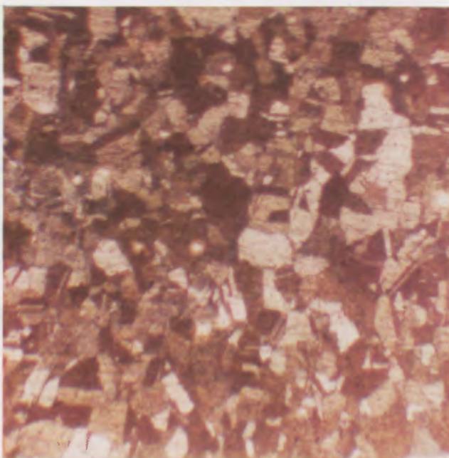
Fig. 25: Same section after reheating, the deformation in the shape of the grains has disappeared. Magnified 100 \times .
