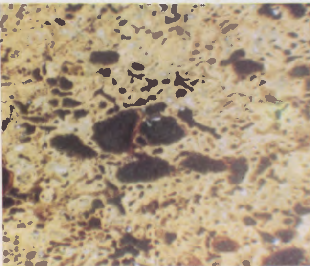
Fig. 48: The same coin. Large black globules of lead distorted by hammering. The blue is phase \delta . Composition c. 8 % Sn, c. 10 % Pb. Magnified 100 \times .
