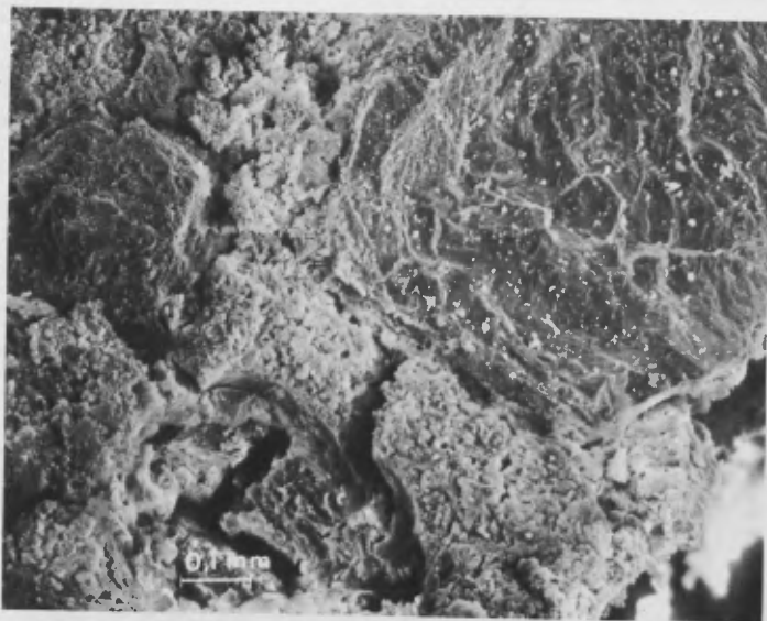
Figure 2 Scanning electron micrograph of the fracture surface of the Erechtheion concrete showing the porous structure left behind after treatment with 1M HCl.
