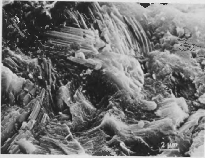
Figure 3 Fracture surface of Caryatid concrete showing \text{Ca}(\text{OH})_2 platelets embedded in CSH-matrix.
