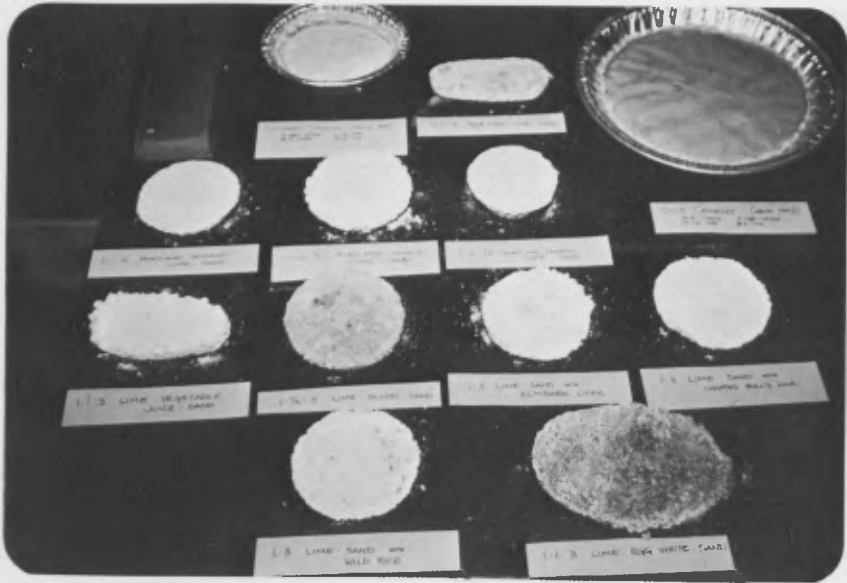
Figure 1: The twelve mortar patties were photographed before testing. Chunam stucco, in the upper left corner, had to be withdrawn from testing as it never solidified.
