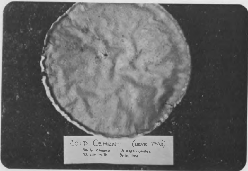
Figure 4: Although ants and ground squirrels showed an interest in the Cold Cement patty, it held up very well under testing. While the surface is irregular, the patty resembles rubber in texture and has excellent plastic qualities.
