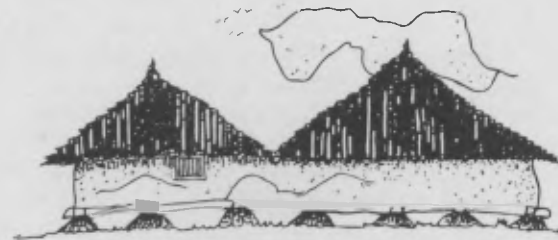
TAMPITA VIHARA - ON STONE BOULDERS MUD STRUCTURE ENCLOSING TIMBER FRAME TILE ROOF.
