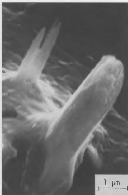
Fig. 27: Lead sulphate conglomerations (detail from Fig. 26)
