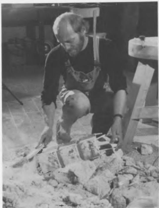
Fig. 20: Preparation of bronze test plates (Foundry at the Master class for sculptures, University of Applied Arts in Vienna)
