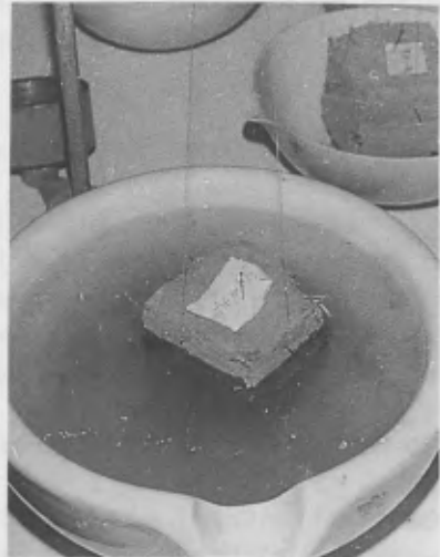
PIC.No.6-7. The laboratory studies made to raise the quality standard of adobe materials. Mimar Sinan University, The Building Materials Laboratory.
