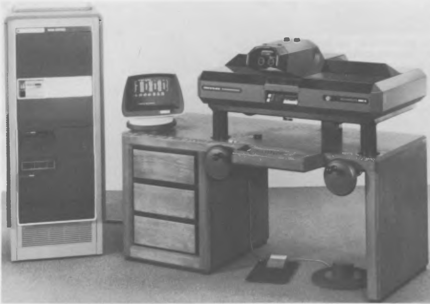
Figure 51 Un restituteur analytique. Aviolyt BC.1 Wild-Heerbrugg. An analytical plotter. Aviolyt BC.1 from Wild Heerbrugg, Switzerland.
