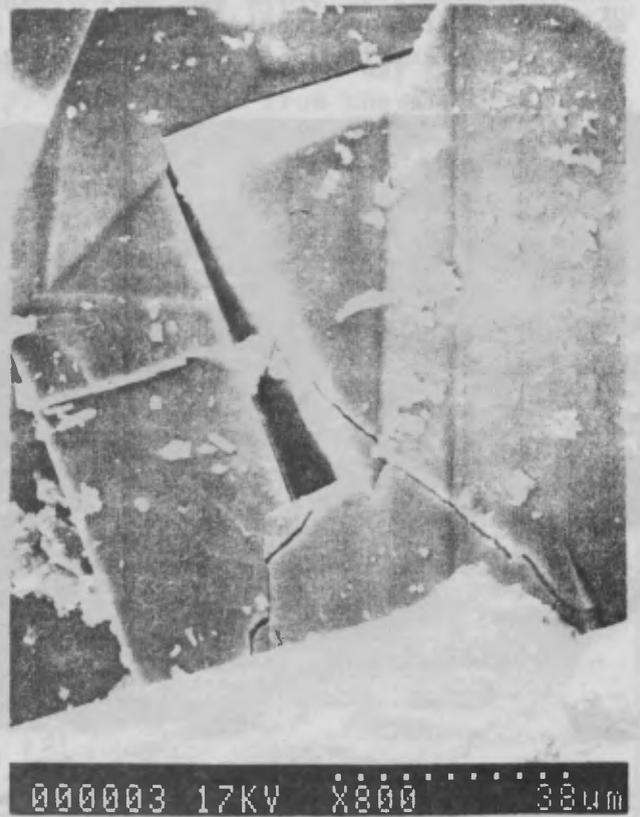
Fig. 12 - (left) Microfractures that tend to spread out towards the external surface of a block of the Tabularium tuff.
