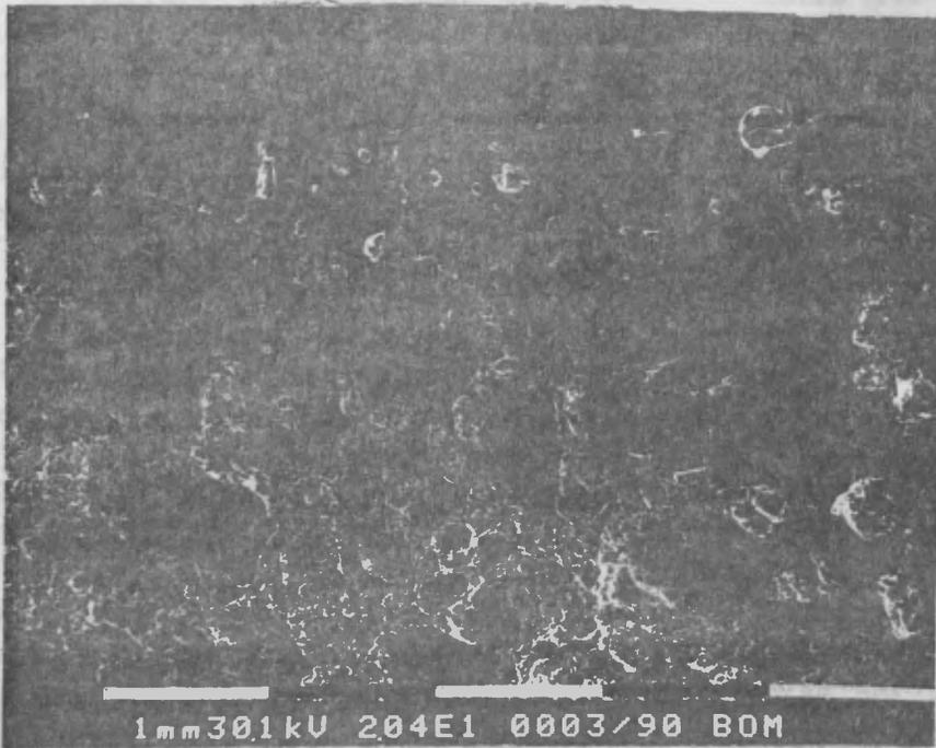
Fig. 8 - SEM microphotography of the patina (20 X). It is possible to see the compact structure and the more homogeneous appearance with respect to the underlying rock.
