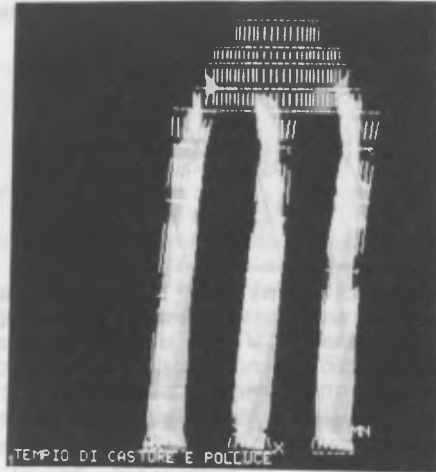
Fig. 3: Numerical model results, longitudinal section: vertical tensions.
