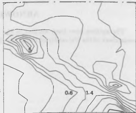
Figure 12: Contours of principal tension stress (as percentage of average compression stress in uniform wall)
