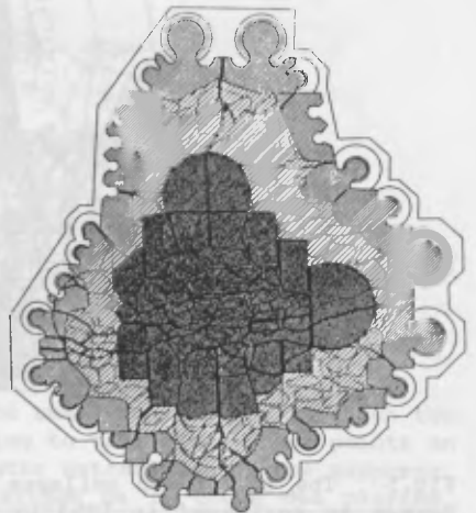
fig.3 Section through a crossing pier of the Cathedral of Bayeux, showing the original Romanesque pier surrounded by later Gothic masonry. (from De Dion, H and Lasvignes, L, Cathedrale de Bayeux: reprise en sous-oeuvre de la tour centrale , Paris, 1861)
