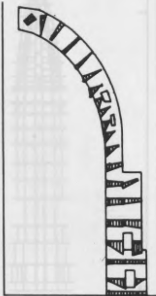
FIG. 8 Meridional compressive stresses at step 10.
