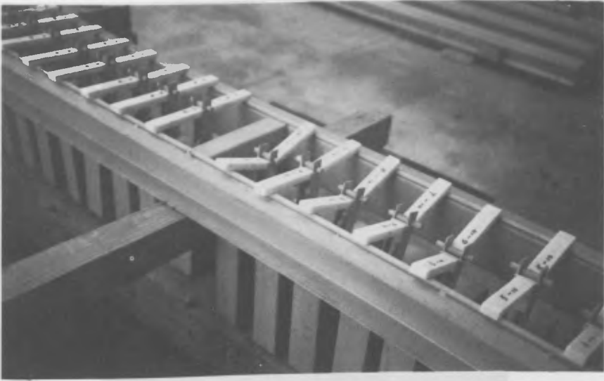
Fig.1 : Bending collapse tests on the marble specimens
