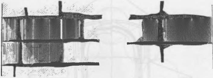
Fig.1 Partial vertical sections through the masonry of a main pier of the Paris Pantheon. (from Rondelet, J, Addition au mémoire historique sur le dome du Pantheon Française , Paris, 1814)
