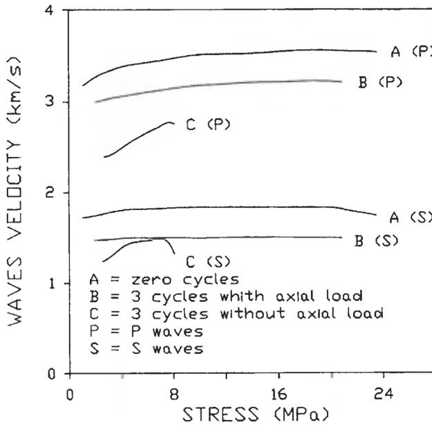
Figure 7.17 Wave velocity for Tabularium tuff samples subjected to salt crystallization tests.
