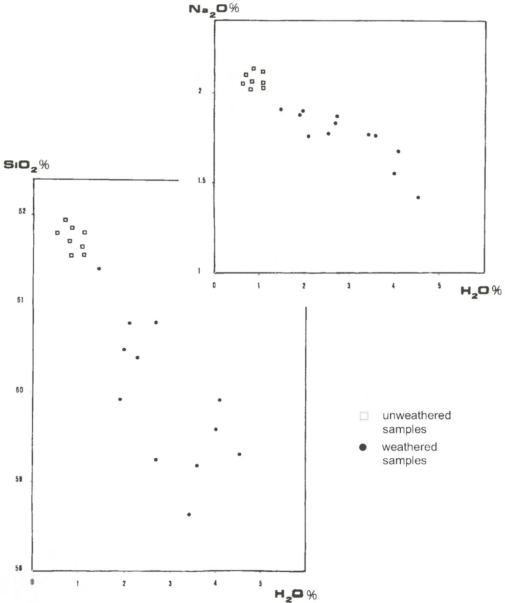
Figure 8.3 Correlation of the concentration of both Na<sub>2</sub>O and SiO<sub>2</sub> with LOI (% H<sub>2</sub>O) for weathered and unweathered specimens.
