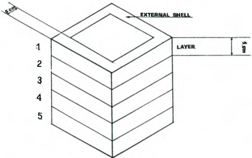
Figure 12.2 The different layers in the original blocks.
