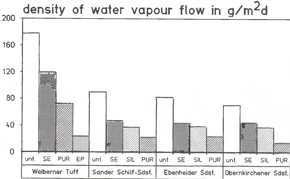
Figure 15.5 Water vapour permeability for treated and untreated stones.
