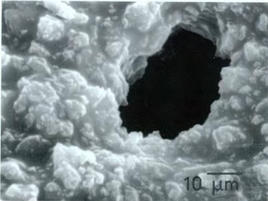
Figure 15.10 - B Internal fracture surface of a tuff sample (WB) after treatment with a PUR-based polymer.
