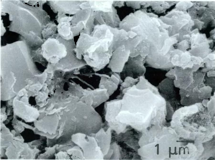
Figure 15.10 - A Internal fracture surface of a tuff sample (WB) before treatment with a PUR-based polymer.
