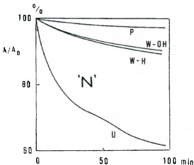
Figure 14.5 Differences in reaction rates with 130 ppm  $\text{SO}_2$ , at 90% RH, for Nara tuff treated with various products. U = untreated; W-H and W-OH = Wacker H and Wacker OH respectively; P = Paraloid B-72.
