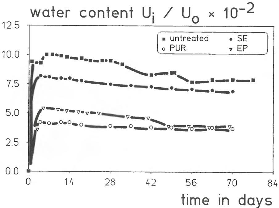
Figure 15.6 Water vapour absorption of treated and untreated tuff (WB) samples exposed to 92% RH at 28°C. The data are given as water content relative to the maximum water absorbed by the untreated sample.
