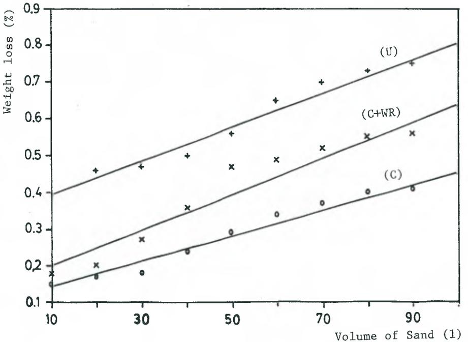
Figure 22.2 Abrasion resistance test for samples weathered by xenotest: untreated (U); consolidated (C); consolidated + water repellent (C+WR)
