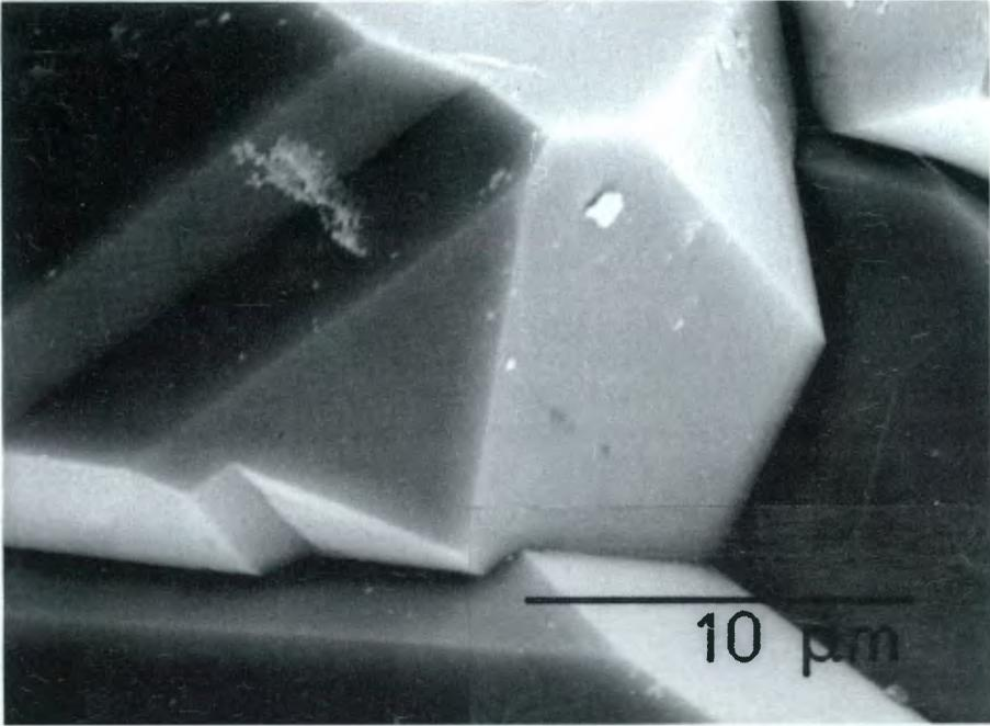
Figure 15.8 - A Quartz crystals in a sandstone (EH) (internal fracture surface) before treatment with an EP-based polymer.
