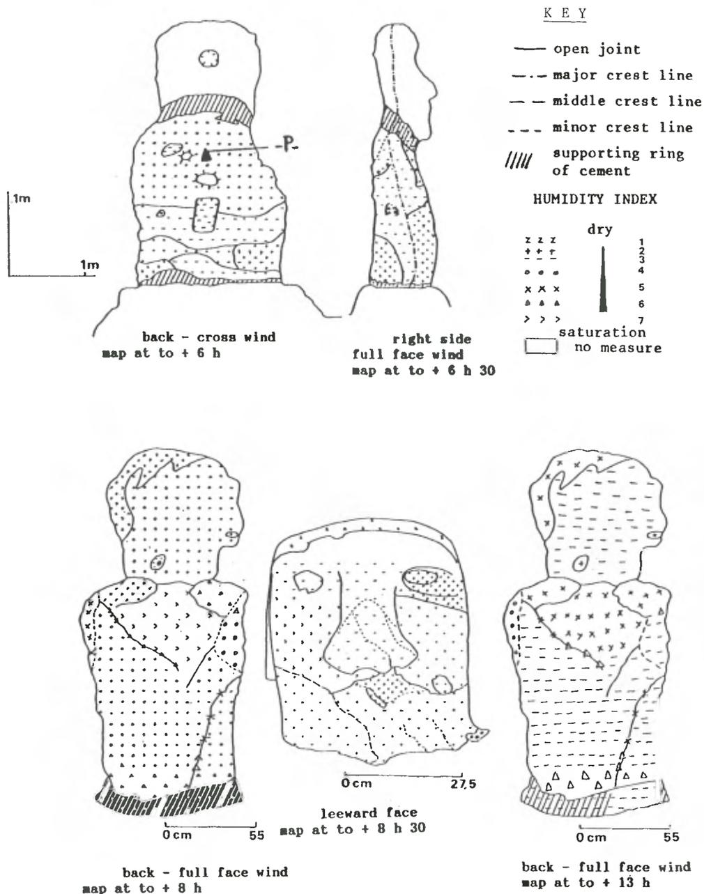
Figure 21.2 Iso-conductance mapping for two moai on Easter Island showing their hydrodynamic behaviour. Top: Hanga Kio'e moai (sample #1) Bottom: moai 4 at Hangaroa (sample #2)  $t_0$  = end of rainfall;  $t_0 + h$  = time at which measurements were taken. P = indicates area from which sample flake was taken.
