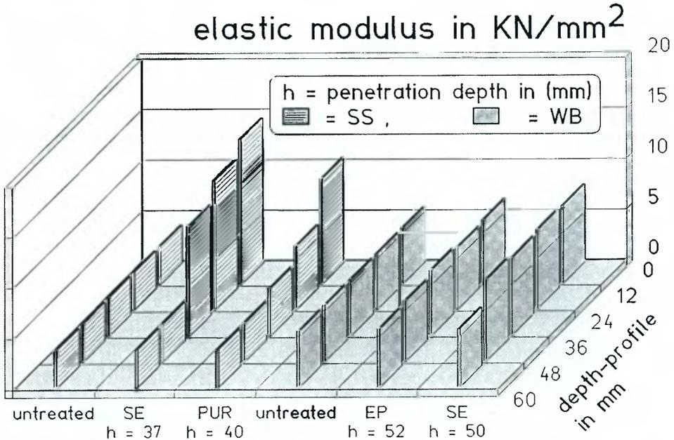
Figure 15.7 Relative elastic modulus depth profiles before and after treatment of sandstone (SS) and tuff (WB) samples.
