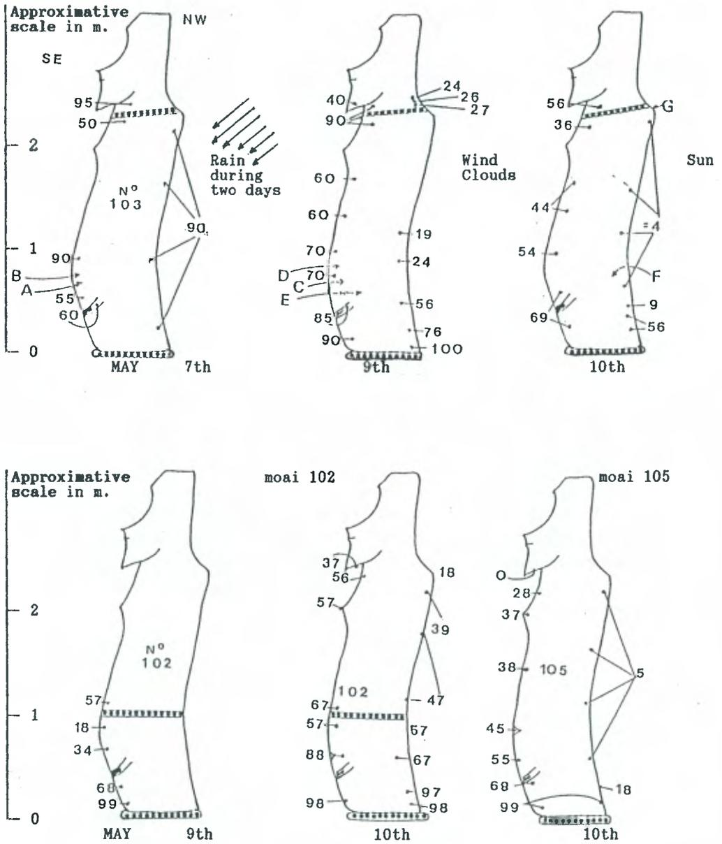
Figure 20.3 Relative water contents, from surface moisture measurements on successive days, in different moai at Ahu Nahunau, Anakena.
