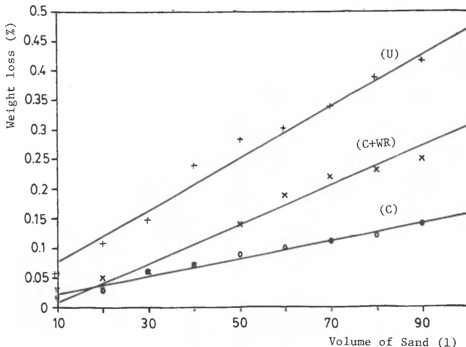
Figure 22.3 Abrasion resistance test for samples weathered by HTOP: untreated (U); consolidated (C); consolidated + water repellent (C+WR)
