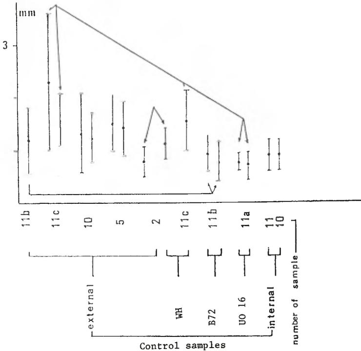
Figure 20.4 Score width on Easter Island tuff samples, untreated and treated with different products. Upper and lower arrows mark results obtained with the same sample.
