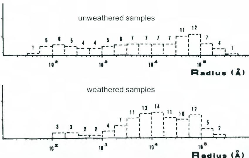
Figure 8.5 Pore size distribution of micropores in weathered and unweathered samples.
