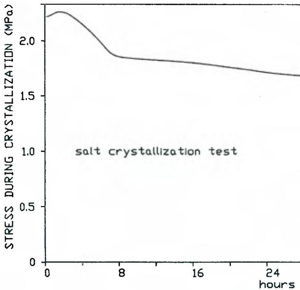
Figure 7.19 Axial stress variation during salt crystallization in the tuff.
