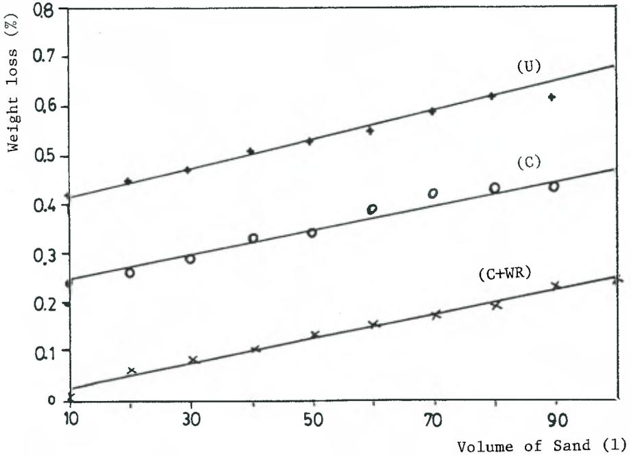
Figure 22.1 Abrasion resistance test for unweathered samples: untreated (U); consolidated (C); consolidated + water repellent (C+WR)
