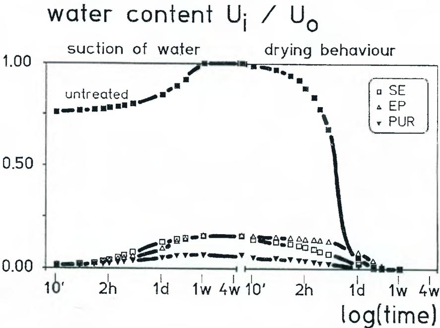
Figure 15.4 Water absorption and drying behaviour of treated and untreated tuff (WB). The results are given as the water content relative to the maximum water absorbed by the untreated sample.
