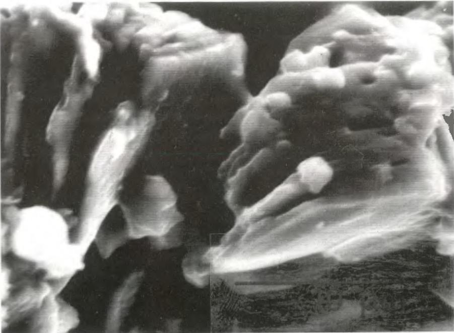
Figure 15.9 - B Characteristic stacks of clays (kaolinite) in a sandstone (OK) after treatment with a PUR-based polymer.
