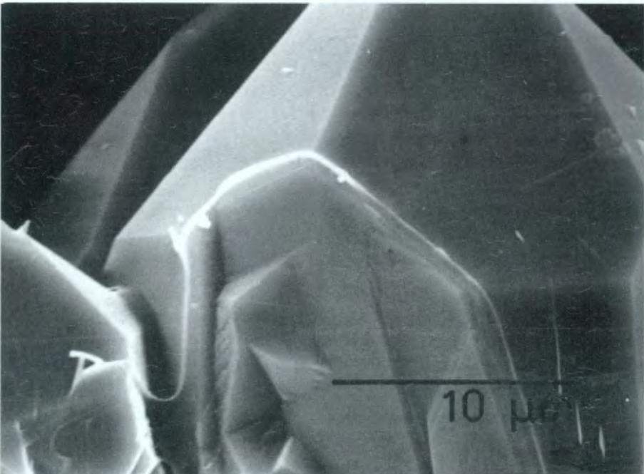
Figure 15.8 - B Quartz crystals in a sandstone (EH) (internal fracture surface) after treatment with an EP-based polymer.
