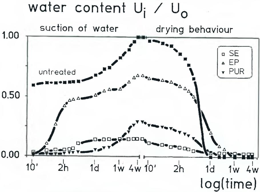
Figure 15.3 Water absorption and drying behaviour of treated and untreated sandstone (EH). The results are given as the water content relative to the maximum water absorbed by the untreated sample.
