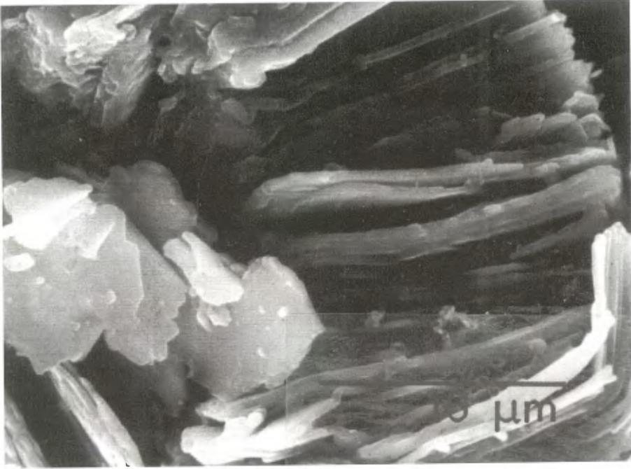
Figure 15.9 - A Characteristic stacks of clays (kaolinite) in a sandstone (OK) before treatment with a PUR-based polymer.
