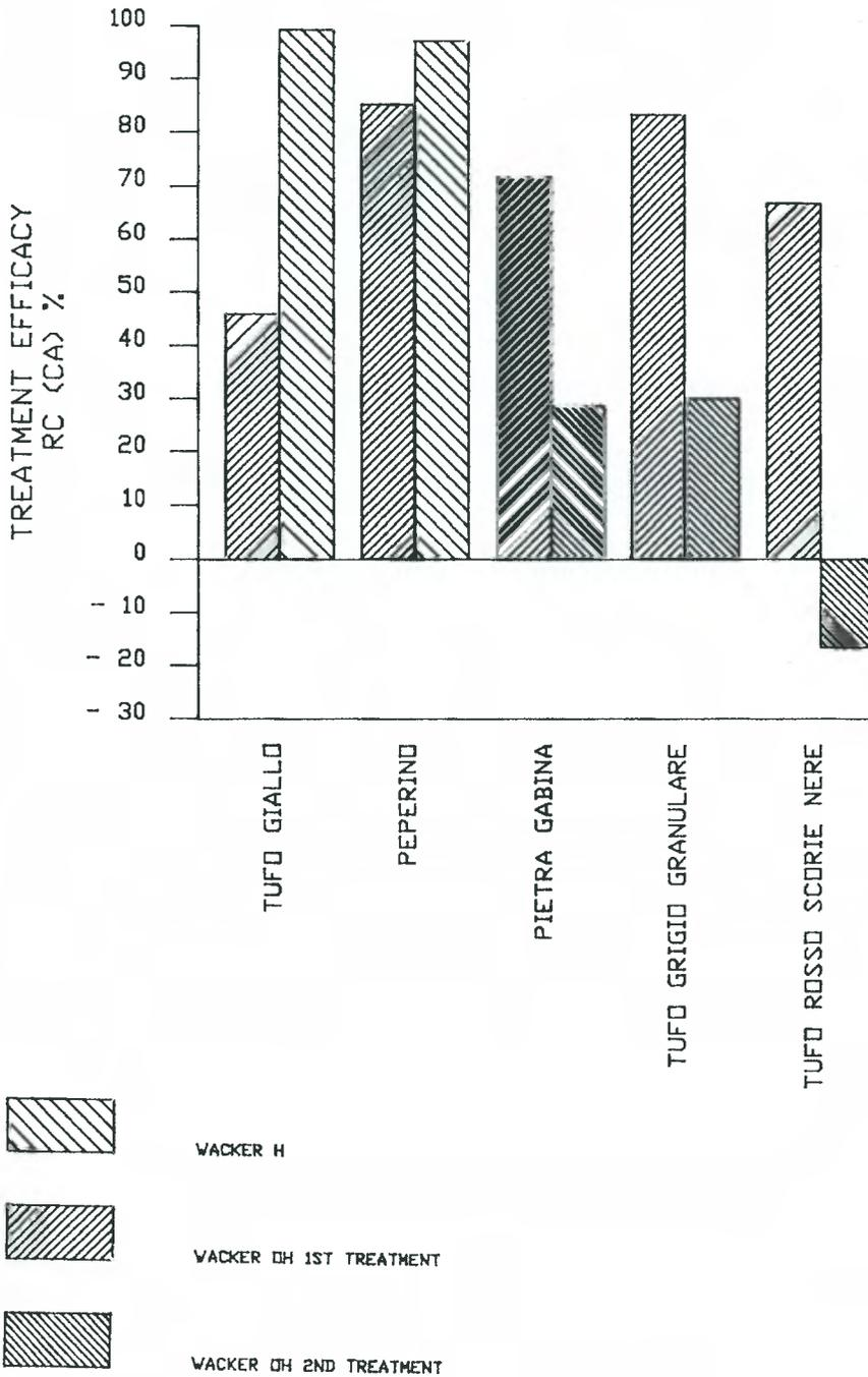
Figure 6.11 Histogram comparing treatment efficacy, based on  $RC_{Ca}$ , for the two treatments studied on different tufts.
