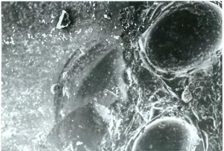
**Figure 3.2** SEM photomicrograph of obsidian after artificial ageing, showing disintegration and alteration occurring around cavities and holes ( $\times 200$ ).
