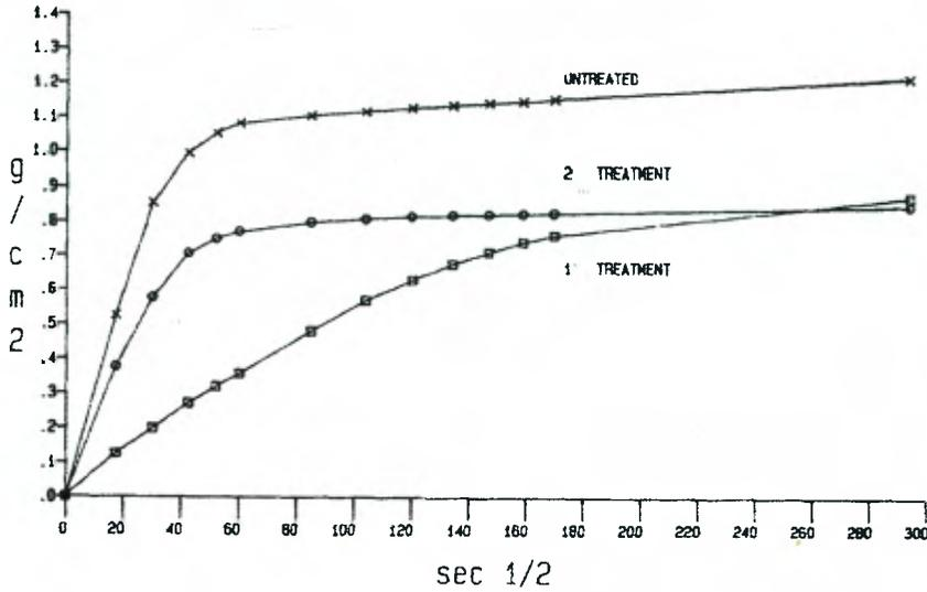
Figure 6.9 Water absorption curves for the untreated and treated samples of Tufo grigio granulare.
