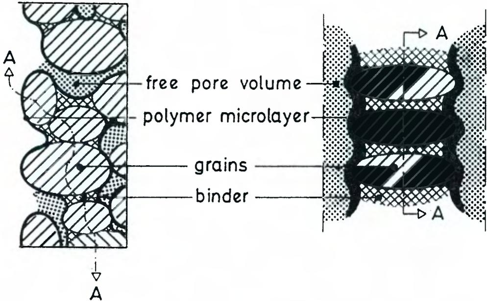
**Figure 15.2** The “supporting corset” protective polymer microlayer coating the pore walls.
