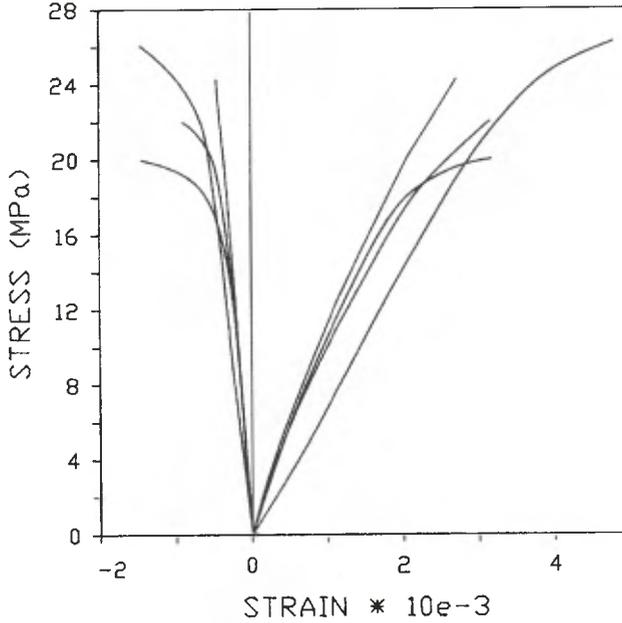
Figure 7.16 Stress/strain diagram for three samples of tuff from the Tabularium and for one sample from one of the Gabii quarries.
