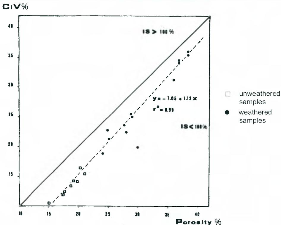
Figure 8.4 Correlation between imbibition coefficient (CiV%) and open porosity. The solid diagonal line represents the 100% saturation index (IS).
