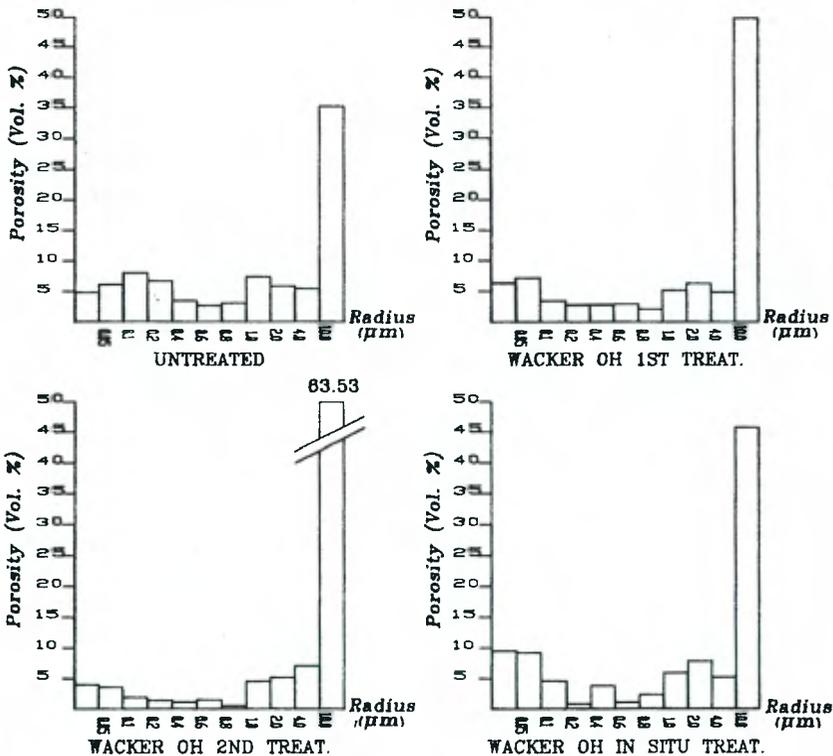
Figure 6.10 Pore size distribution histograms for the untreated and treated samples of Tufo grigio granulare.
