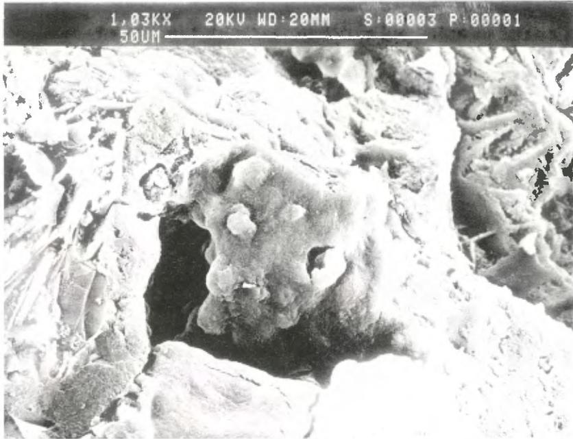
Figure 23.3 SEM photomicrograph of a fracture surface. The area shown was approximately 0.2 mm below the surface treated with *BSM 100 W*. Note the uncoated, platelike minerals on the left side of the photograph.
