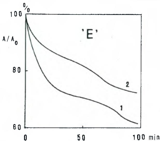
Figure 14.4 Influence of RH on the corrosive action of 150 ppm  $\text{SO}_2$  on Echizen tuff. Curve 1 = 90% RH; Curve 2 = 75% RH.
