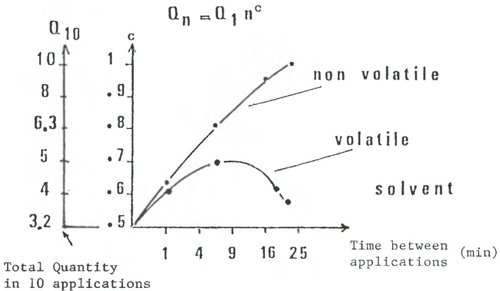
Figure 20-B.1 Influence of the solvent on the relationship between penetration index and the time between applications.
