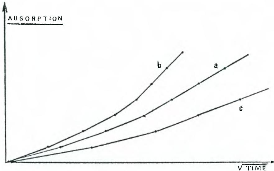
Figure 20.2 Water absorption curves for a tuff sample with different amounts of moisture: (a) dry, i.e., in hygroscopic equilibrium; (b) damp, i.e., water content about 30%; and (c) wet, i.e., water content above 40%.
