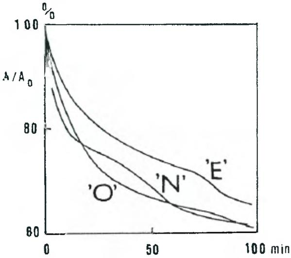
Figure 14.2 Relative decrease in radioactivity for the three tuffs in a corrosive atmosphere of 125 ppm  $SO_2$  at 85% RH. O = Oya; N = Nara; and E = Echizen tuff.
