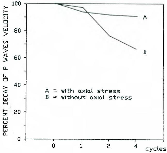
Figure 7.18 Wave velocity decay with and without axial stress for Tabularium tuff samples.
