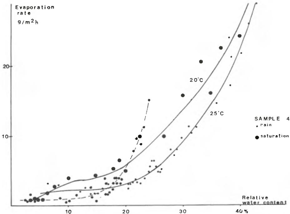
Figure 20.1 Comparative drying curves for a coarse-grained sample (N° 4) wetted first by rain and, in a second experiment, by saturation. Also included is the drying curve for a fine-grained sample (N° 1) wetted by rain.
