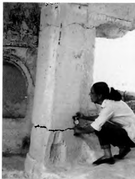
Figure 11. Use of a removable mechanical strain gauge for measuring the movements of a crack in a pillar of El Nazar.
