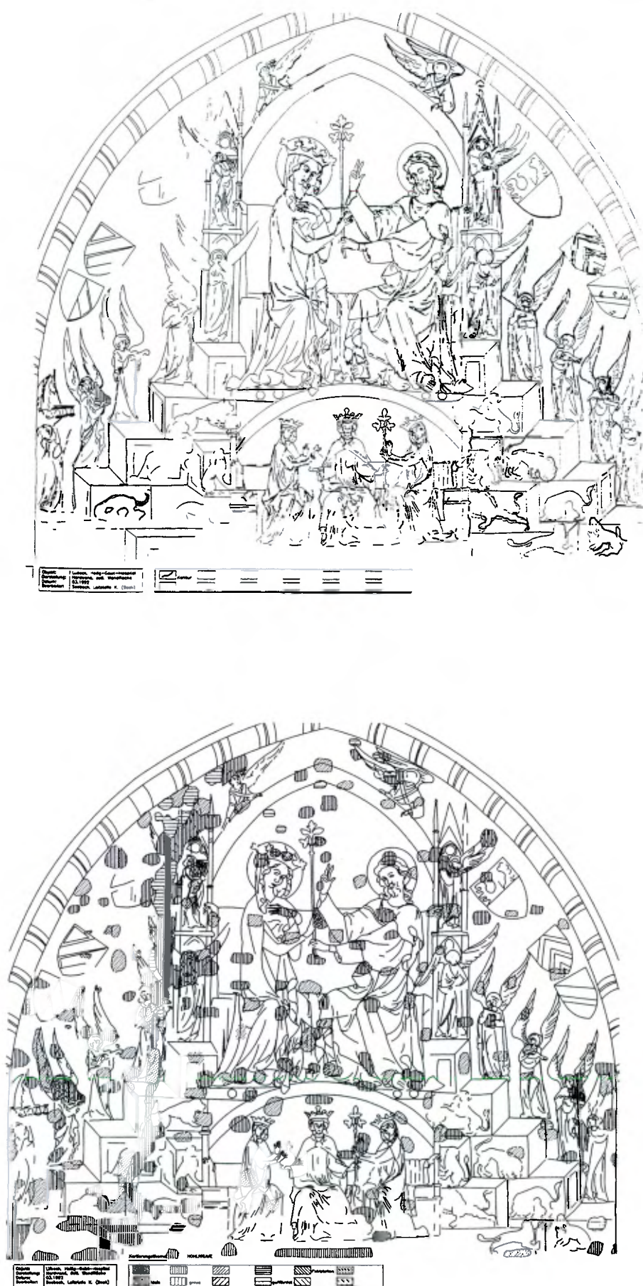
Figure 5. Above: Overview of flaking contours. Below: Distribution of gaps and lack of adhesion.
