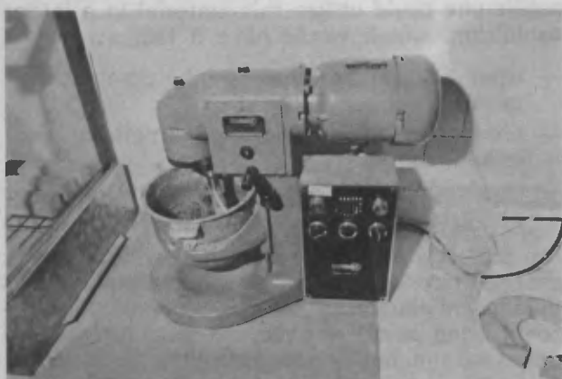
18 The mortar is prepared in a special heavy-duty mixer.
