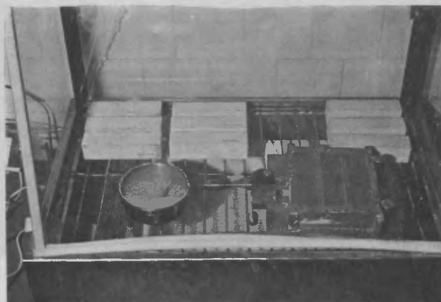
The samples are cured in a humid cabinet at a constant temperature and relative humidity.
