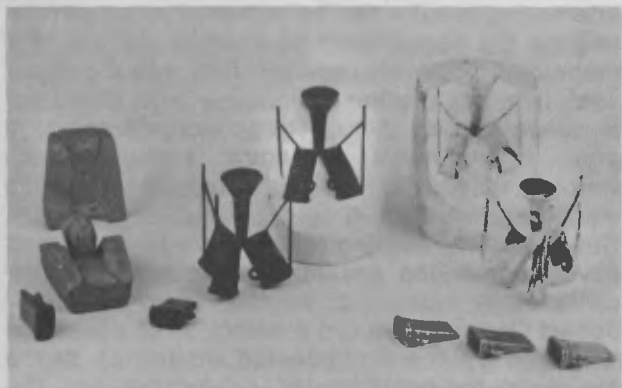
Models demonstrating the lost-wax casting process. From left: wooden pattern, clay mould for making waxes, wax model, section through invested waxes, investment section after burnout, casting removed from investment, and finishing stages. Photo by B. Malter.
