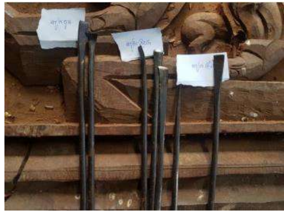
Fig 33b. Leas Chok, Leas Krachak, Leas Trang (Chisels of shell shape: scoop, nail, and straight)
