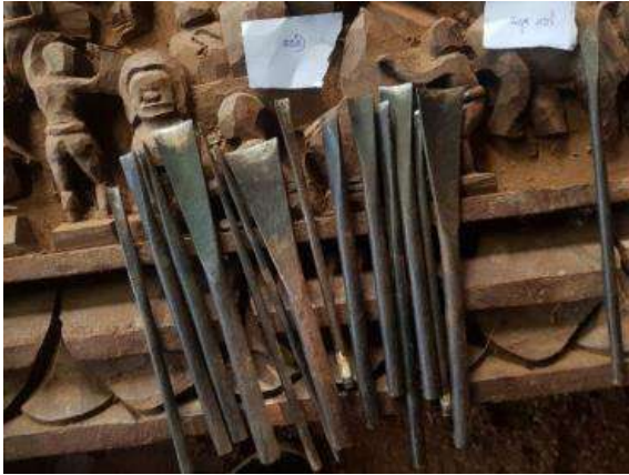
Fig 33a. Ponleak Krachak and Dek Svan (Chisel of nail shape and drilling tool)
