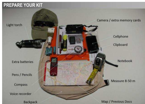
Figure 5. Basic kit for emergency documentation. Such kits were constructed during the courses. An important aspect of this was to have backup documentation tools, techniques and systems (Eppich and Almagro Vidal, 2013).
