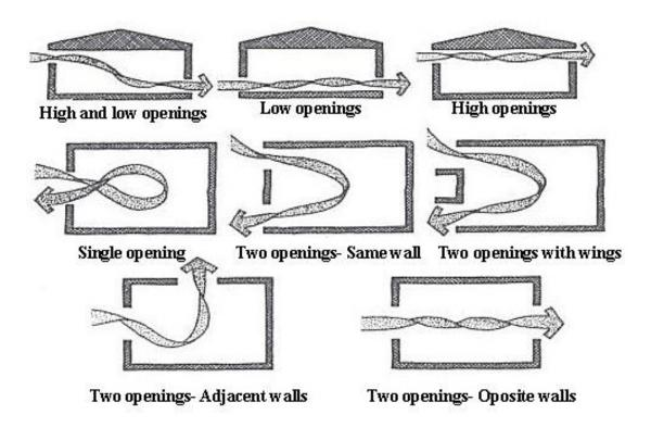
Fig. 2- Different types of natural ventilation in buildings.
