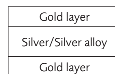
FIGURE 2 Layer structure of the double-sided gilt silver strip
